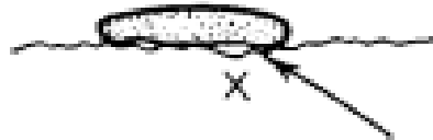
Figure 2.6 An illustration of good and poor wetting by an adhesive spreading over a surface. 9
